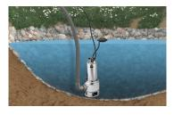
Submersible pump for waste water and drainage applications. BIOX 300/10 is a professional pump with a stainless steel pump body, motor shaft, impellers and pump base, allowing to leave the pump permanently in water without any risk of corrosion. High realibility thanks to the vortex impeller.
